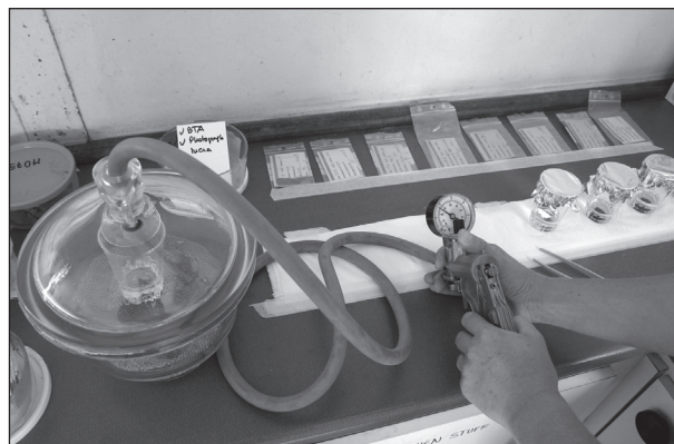
36. Chemical and physical stabilization is performed under vacuum. © IJP_Brahe.
